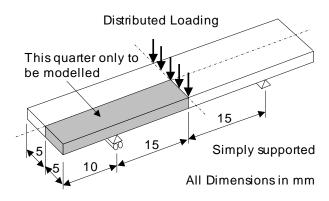
A 50mm x 10mm x 1mm thick composite strip, composed of an 8-layer composite material is to be analysed first using shell elements and then using solid elements in order to compare the results obtained.
