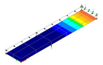
laminate 1 (as shown on the contour key) is only 0.26 so no failure has occurred due to the applied loading.
