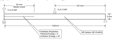
The model is required to predict the growth of a crack within a unidirectional composite laminate subjected to mixed-mode loading. A starter crack 30 mm long is introduced at one end of a double cantilever beam (DCB) specimen. A tensile (crack opening) load is applied to the cracked end of the sample while a compressive (crack closing) load is applied to the centre of the specimen. The resulting delamination crack propagates along the length of the sample under mixed-mode conditions.
