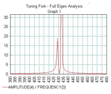
This displays a better representation of the displacement/ frequency response in the vicinity of the first two mode shapes.
