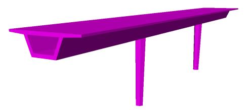
The bridge consists of a 3-span reinforced concrete deck of box section. The central span is 25m and the end spans are 14m. A pier is provided at each end of the central span. The piers are 6m high, hexagonal in shape and tapered. The concrete is grade C40/50 and the reinforcement is grade 500B throughout. Vertical support is provided at each end of the bridge. To concentrate on the definition of beam reinforcement and frame design no diaphragms in the deck are modelled.
