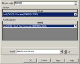
Back on the RC Material dialog enter the name as Reinforced Concrete and click OK.
