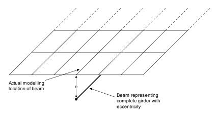
Beam element modelling of the whole girder
