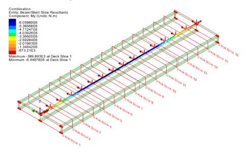
**Note.** The size of the drawn slice plane depends upon the elements that are sliced. By default, slice planes and local slice axes are drawn in red, but these and other visualisation settings relating to slice axes, slice planes and slice labels can be specified from the Utilities layer properties dialog, which is accessed from the Utilities  $\sqrt{2}$  treeview.
