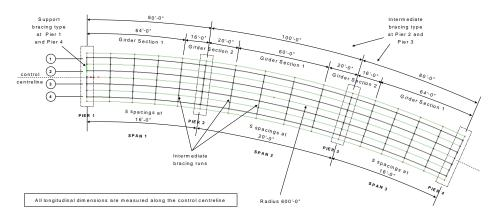
The bridge consists of three spans of length 80 feet, 100 feet and 80 feet. The bridge follows a radius of 600 feet along the control centreline and all supports are along
