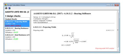
It can be seen that, for both stiffener types, the Projecting Width check is not satisfied. This can be resolved by increasing the thickness of the stiffeners. This is covered at the end of the example.
