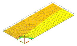
The contour key should be showing a maximum stress in the lamina X material direction of around 1.8E3
