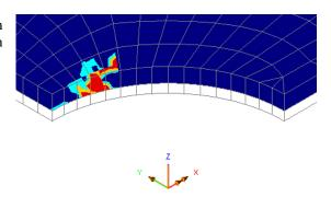
• By changing the active loadcase it can be seen that no failure has occurred after the first load increment (a load factor of 0.5). By the second load increment (a load factor of 0.75) a small amount of matrix failure has occurred adjacent to the hole.
