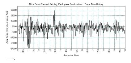
Peak results for the averaged element forces and moments are displayed in Notepad in file peak\_forceSet\_Avg1.sum. These indicate a peak positive average axial (Fx) force of 32.7kN at solution time 0.98 seconds and a peak negative average axial (Fx) force of -36.1kN at 1.01 seconds for the 1940 El Centro earthquake (Record 1), as shown in the following figure.
