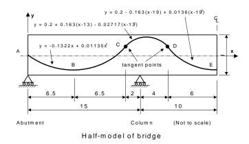
The initial post tensioning force of 5000 kN is to be applied from both ends. Tendons with a cross section area of  $3.5e3mm^2$  are located every 2 metres across the section allowing the analysis to model a 2 metres effective width.
