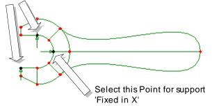
• Click the **OK** button to assign the support to the Point selected for all the loadcases in analysis 1.
