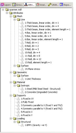
The spanner will be meshed using both regular and irregular Surface meshes. A regular mesh is to be used for the jaws of the spanner. An irregular mesh will be used for the handle.
