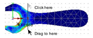
Utilities Graph Through 2D... • Ensure that Loadcase 1 and an extent of Visible model are selected, and Click the Next button.
