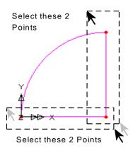
Using the New Surface button, create a Surface from the Lines selected.
