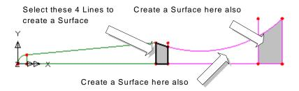
• Select the 4 Lines (remembering to hold the **Shift** key down after the first line is selected to add to the selection) to form the boundary of the Surface shown.
