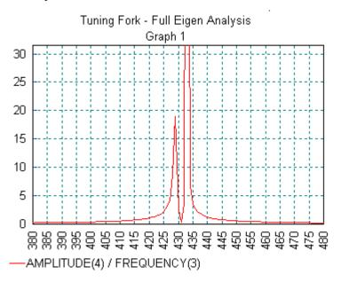
This displays a better representation of the displacement/ frequency response in the vicinity of the first two mode shapes.
