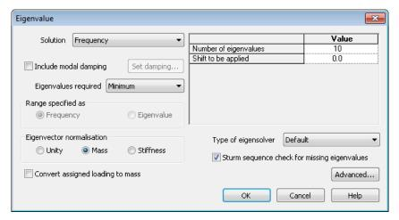
The following parameters need to be specified to perform a frequency analysis with a specified number of the minimum eigenvalues.
