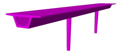
The bridge consists of a 3-span reinforced concrete deck of box section. The central span is 25m and the end spans are 14m. A pier is provided at each end of the central span. The piers are 6m high, hexagonal in shape and tapered. The concrete is grade C40/50 and the reinforcement is grade 500B throughout. Vertical support is provided at each end of the bridge. To concentrate on the definition of beam reinforcement and frame design no diaphragms in the deck are modelled.
