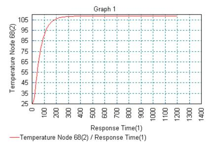
From the graph it can be seen that the outside of the pipe reaches its steady state condition after approximately 300 seconds.
