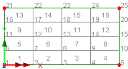
Before: All nodes and elements numbered using global directions.
