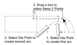
• Thirdly, drag a box around the two unconnected Points at the top of the model.
