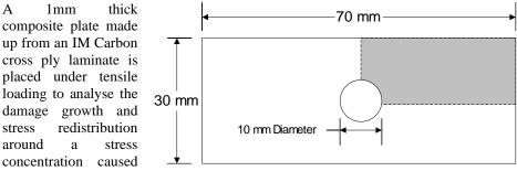
by a 10mm diameter hole. Because of symmetry a quarter model will be created.
