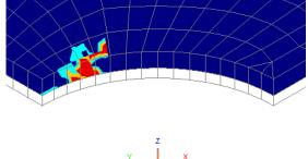
• By changing the active loadcase it can be seen that no failure has occurred after the first load increment (a load factor of 0.5). By the second load increment (a load factor of 0.75) a small amount of matrix failure has occurred adjacent to the hole.
