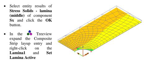
The contour key should be showing a maximum stress in the lamina X material direction of around 1.8E3
