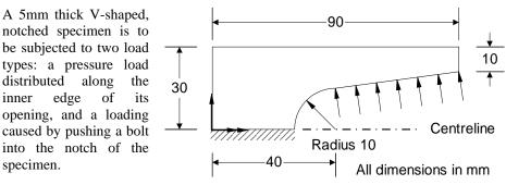
After an initial linear analysis with the specimen subjected to the pressure load, nonlinear material properties are defined, and a nonlinear analysis is carried out using the same pressure loading.
