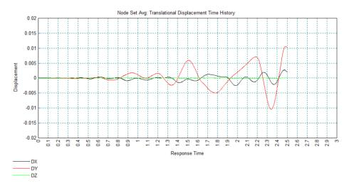
The peak results for the averaged node displacements are displayed in Notepad in file **peak\_dspSet\_Avg1.sum**. These indicate absolute peak average displacements of 0.0027m at time 2.4725 seconds in the X-direction and 0.0106m at time 2.485 seconds in the Y-direction.
