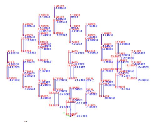
• In the  $\bigcirc$  Treeview right-click on the Whole Earthquake (Max) envelope and select the Set Active option to set this envelope active. Select entity Force/Moment of component My. Ensure that Change existing drawing layers to above component is selected, then click the OK button.
