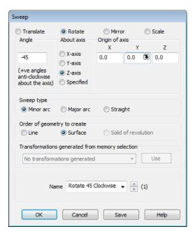
Whilst a suitable line on this newly created surface could be swept to create another surface, instead the surface just drawn be copied to achieve the same result by rotating it through a 45 degree rotation clockwise.
