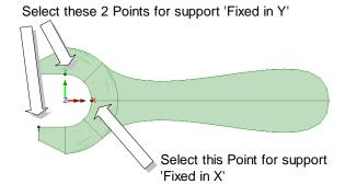
• Click the **OK** button to assign the support to the Point selected for all the loadcases in analysis 1.
