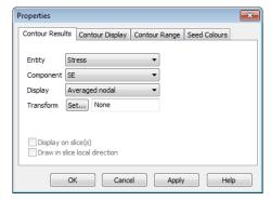
Click the OK button to display the contour plot of equivalent stress along with the contour key.
