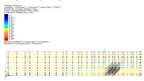
• Click **OK** to update the display and show the actual crack width value calculated at gauss points within the element.
