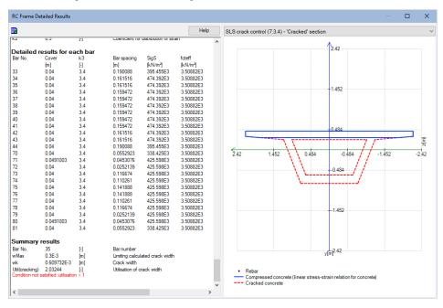
Under the 'Detailed results for each bar' heading the bars for which the crack width check has been applied are listed. The location of these bars (bars 33-44 and 70-81) can be found under the 'Section Definition' 'Reinforcement' heading further up the listing, which shows most of the bars to be in faces 6 and 11 (the lower and upper faces of the bottom of the box section).
