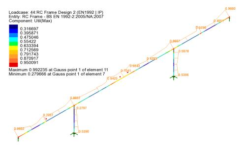
From this diagram the peak Utilisation value in the deck can be seen to be **0.992** as previously obtained.
