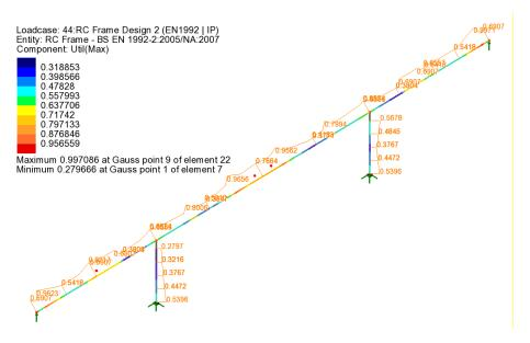
When compared to the values that previously passed the initial design check, an increase in the maximum utilisation in the central and end spans is seen.
