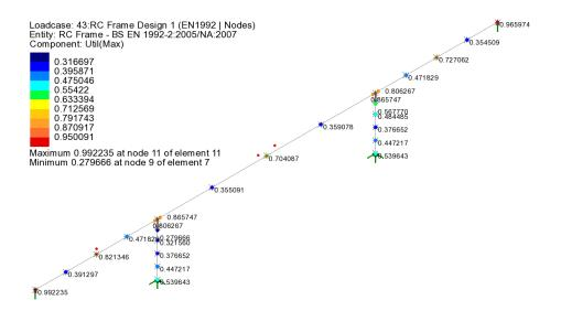
Utilisation values are now all less than 1.0 with the largest value of **0.992** occurring in the deck. Whilst the reinforcement used has not been optimised, the bridge has effectively passed the design check.
