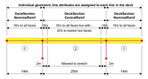
For each section reinforcement utility, the following bar diameters are defined for the faces stated:
