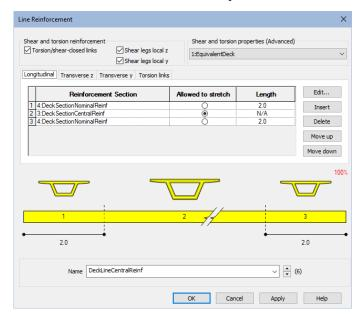
The central region is un-dimensioned and would be 'Allowed to stretch' to fit the remainder of the length of this span.
