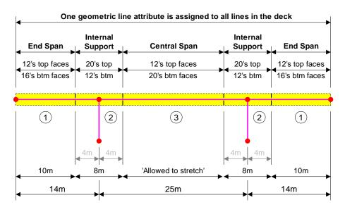
For each section reinforcement utility, the following bar diameters are defined for the faces stated.
