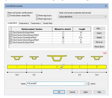
Note that the central span region is un-dimensioned and is 'Allowed to stretch' to fit the length of the deck that remains between the support regions.
