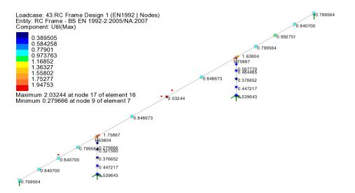
From the nodal results it can be seen that the utilisation values exceed 1.0 in the deck at both pier supports and also in the central span. Results for these locations will require further investigation. Utilisation values in the piers are less than 1.0.
