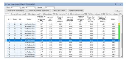
• Scroll down the table and select the first entry for the pier (this should be Line 6 Element 8 Node 10) and then click the **Detailed results for selected row** button at the top of the dialog.
