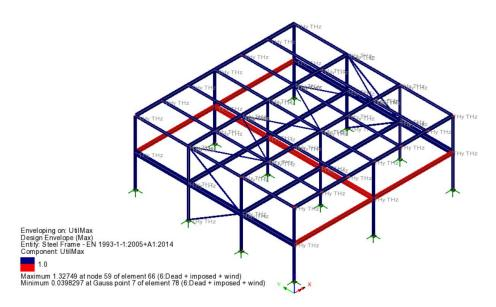
The Design contour option is useful to see members that fail but also to get an indicative quantification of the utilisation of members that pass the design checks. Members with a low utilisation (less than 70%) are not contoured. To activate this appearance:
