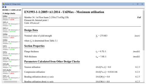
From the Design Check Summary report it can be seen that by scrolling to the bottom of the report the maximum utilisation factor of 1.32749 is obtained from the Util(Fx\_c,My,Mz,b) design check.
