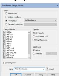
On completion a 'First floor beams' entry is created inside the Steel Frame Design Results folder in the Utilities treeview.
