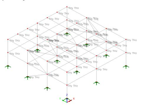
Toggling the Fleshing button on and off will show the steelwork arrangement.
