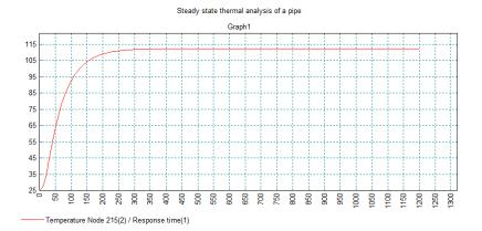
From the graph it can be seen that the outside of the pipe reaches its steady state condition after approximately 300 seconds.
