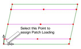
• Enter the loadcase as Lane load (lower) with a load factor of 1 and click OK
