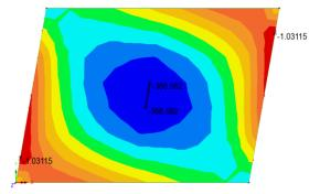
moment MY(B) equals the capacity of the slab MY\*(B). This would result in a restriction in the load carrying capacity of the slab.
