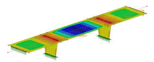
This shows that the bending moment at the location of the bearings (joints) of the dropin span is zero as the joints don't have any rotational stiffness.
