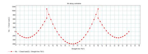
By hovering the cursor over graph points of interest it can be seen that the peak moment at the internal supports in 1092kNm and the lesser moment is 654kNm – meaning that the pier is currently attracting a moment of 1092 - 654 = 438kNm.
