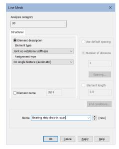
• In the model view window select the **6 lines** that define the extent of the drop-in span.
