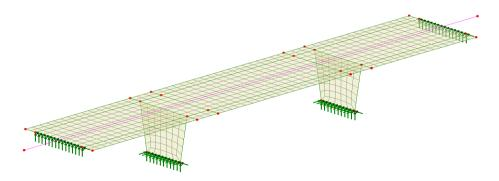
Groups have been defined for the features in the deck and the piers. These are used to restrict the extent of data used to create graphs of results along the deck. The line along the centre of the bridge is used when graphing results.
