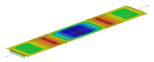
This shows that the moment along the lines of the bearings (joints) of the drop-in span is zero as the joints don't have any rotational stiffness.
