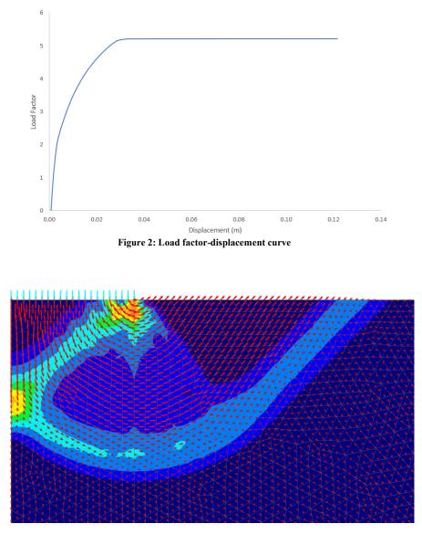
Figure 3: Displacement vectors – effective strain contours
