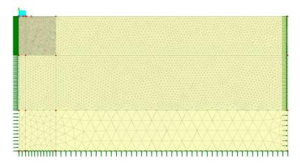
Figure 1: Finite element mesh showing supports.
