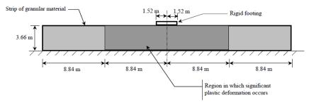
Figure 1: Dimensions of the granular material for which the limit load analysis is carried out. The dark shaded area is considered the region where significant plastic deformation takes place.
