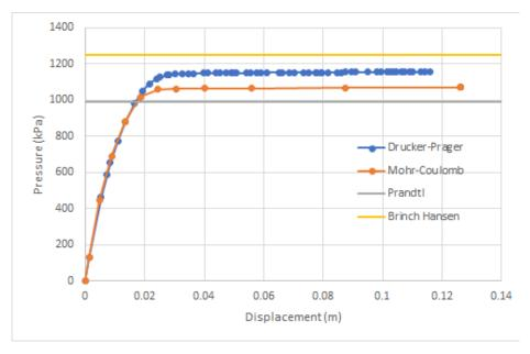
Figure 3: Variation of pressure underneath the footing against applied displacement
