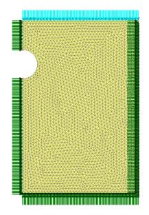
Figure 1: Finite element mesh showing supports.
