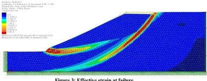
Figure 3: Effective strain at failure
