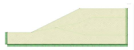
Figure 2: Mesh and boundary conditions
