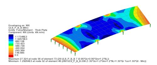
From the Contour key minimum values occur in combination 280: ULS\_P 258 (1.35\*Gc+1.2\*Grs+1.2\*SL+1.35\*Qt Tch-Min).
