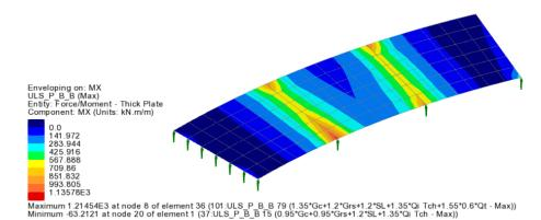
From the Contour key it can be seen that maximum values occur in combination 101:ULS P B B 79 (1.35\*Gc+1.2\*Grs+1.2\*SL+1.35\*Qi Tch+1.55\*0.6\*Qt - Max).
