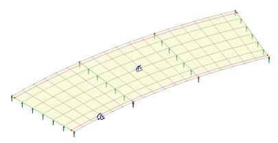
The structure is modelled using thick plate elements, representing a deck of inner radius 75m, outer radius 86m and thickness 0.7m. The deck has a width of 11m consisting of a 10m wide carriageway region and two 0.5m wide verges.
