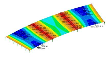
The structure is modelled using thick plate elements, representing a deck of inner radius 75m, outer radius 86m and thickness 0.7m. The deck has a width of 11m consisting of a 10m wide carriageway region and two 0.5m wide verges. The live loading is to be calculated for three defined influence surfaces using the LUSAS VLO software option.
