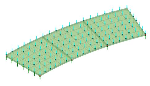
In the D Treeview, using the right-hand mouse button, select Loadcase 1 and select the Rename option. Change the loadcase name to Self Weight
