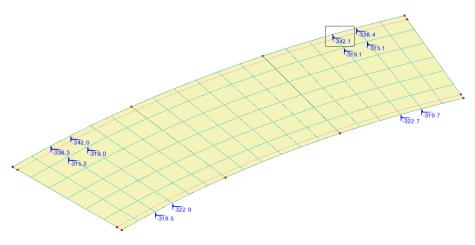
• Select node 106, then, for the active loadcase, select the context menu item Visualise loading at node. The load pattern causing the effect at that location will be drawn on the model and the loading details displayed in the Analyses  $\bigcirc$  treeview.
