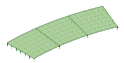
The structure is modelled using thick plate elements, representing a deck of inner radius 75m, outer radius 86m and thickness 0.7m. The deck has a width of 11m consisting of a 10m wide carriageway region and two 0.5m wide verges. The live loading is to be calculated for whole structure the LUSAS VLO software option.
