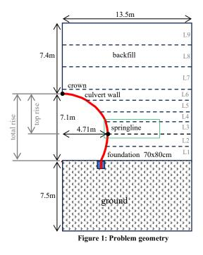
This analysis considers the construction of a long-span arch culvert from curved corrugated metal with ends anchored in concrete footings. Backfill soil is compacted
