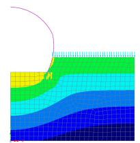
Figure 7: Vertical stresses after compaction of first layer
