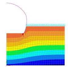
Figure 7: Vertical stresses after removal of compaction load
