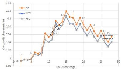
Figure 8: Variation of crown displacement with loading
