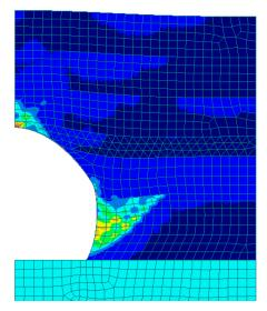
Figure 10: Effective plastic strain at end of loading
