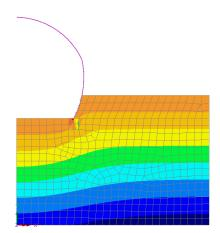
Figure 6: Vertical stresses after first backfill layer is activated
