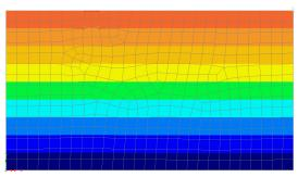
Figure 4: Initial vertical stress distribution in ground
