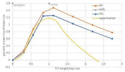
Figure 9: Displacement of crown with increasing backfill
