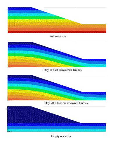
Figure 9: Pore water pressures for reservoir in different states
