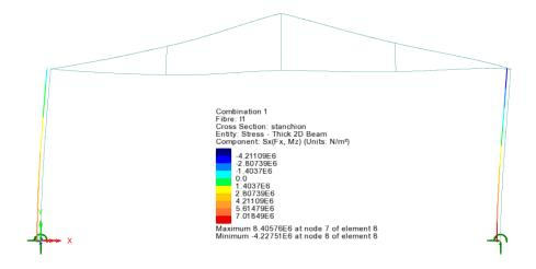
Initially the contours of stress will be drawn only at the current active fibre location on both stanchions as seen on the image above. A contour key will also be drawn stating the maximum and minimum values for this fibre location. Fibre locations will be explained shortly.
