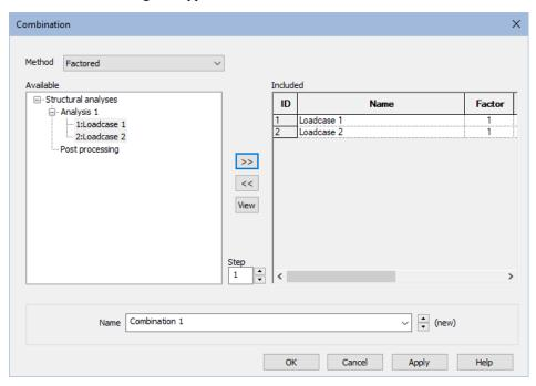
Both available results loadcases should be added to the Included combination panel.
