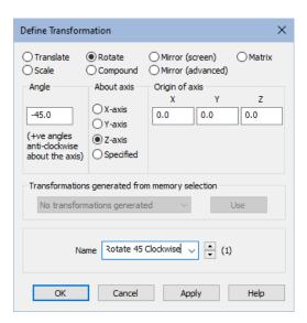
Whilst a suitable line on this newly created surface could be swept to create another surface, instead the surface just drawn will be copied to achieve the same result by rotating it through a 45 degree rotation clockwise.
