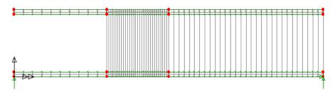
• Select the point at the bottom left-hand corner of the model, drag and drop the support attribute **Fixed in Y** onto the selection and click **OK** to assign to Points.
