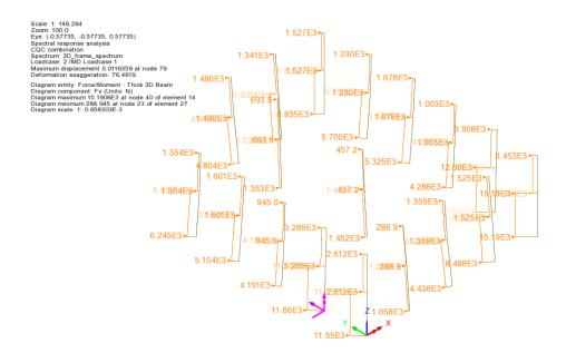
Results will be calculated for the active IMD load case and an axial force diagram of force in each member will be displayed. If necessary, use the Zoom in button to view results information. These types of results can also be plotted in isolation on selected model features.
