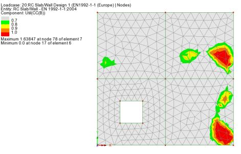
From this it can be seen that the Util(CC(T)) is critical over the central column support while Util(CC(B)) is critical in the span near the right hand edge of the slab.
