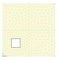
In this manner the mesh density on slabs can be varied according to the levels of detail required.
