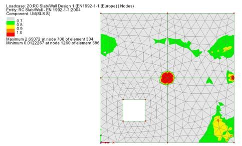
Further contour plots are available which can provide additional information. For example the plot of Util(CC) can be separated into top and bottom checks, Util(CC(T) and Util(CC(B)) receptively as shown below.
