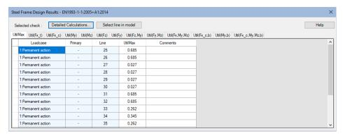
If the 'Detailed Calculations' button were pressed for a selected row, steel frame design results could be added to a model report by using the 'Add to report button' on the results dialog, but for this example this will not be done. Instead, steel frame design summary results will be added to the model report using the reporting facility directly.
