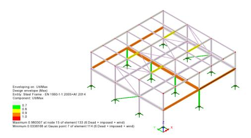
So it can be seen that, for this example, the illustrative results obtained by assigning revised section properties to a previously solved model very closely match the actual results obtained from re-solving the model using those revised properties.
