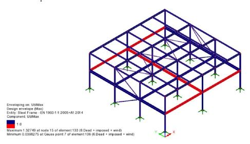
The Design contour option is useful to see members that fail but also to get an indicative quantification of the utilisation of members that pass the design checks. Members with a low utilisation (less than 70%) are not contoured. To activate this appearance:
