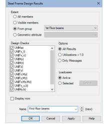
On completion a 'First floor beams' entry is created inside the Steel Frame Design Results folder in the Utilities treeview.
