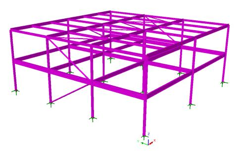
The frame consists of hot rolled structural steel sections, steel grade S 275, hot finished hollow sections, steel grade S 355 H and user-defined grade hollow section.
