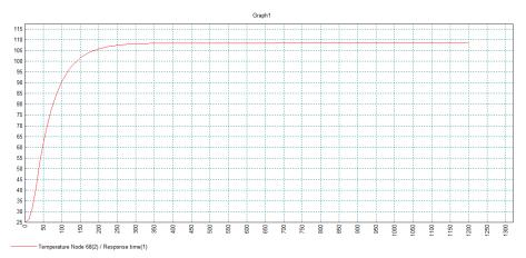
From the graph it can be seen that the outside of the pipe reaches its steady state condition after approximately 350 seconds.
