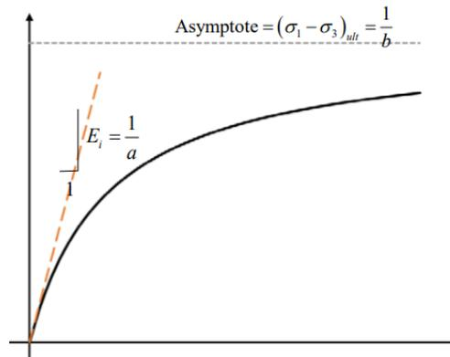
Figure 2: Hyperbolic stress-strain curve
