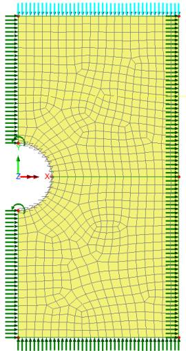
Figure 2: Finite element mesh showing supports and load
