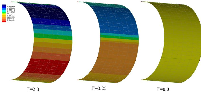
Figure 8: Contours of shear stress on interface of 3D model
