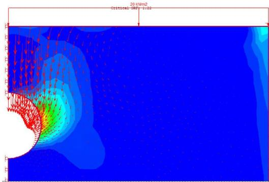
Figure 5: Maximum Shear Strain in RS2 [2]
