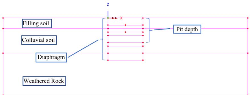
Figure 3: Model geometry
