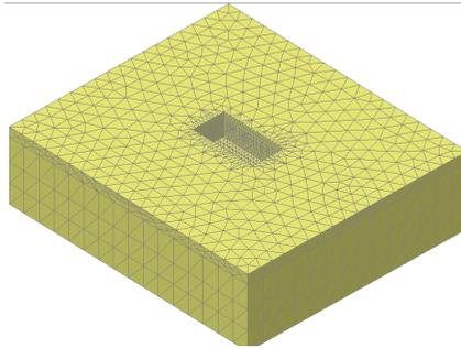
Figure 8: Model mesh of excavation
