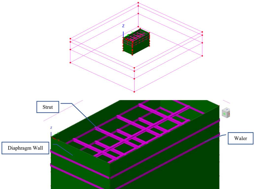
Figure 2: Structural elements
