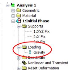
Figure 12: Adding gravity to the model
