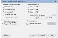
Note that a single special vehicle (SV1800200low) is specified as a default in these recommended values and that a vehicle(s) appropriate to the structure being designed should be specified in practice.
