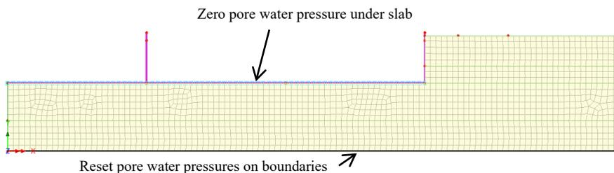
Figure 7: Boundary conditions for dissipation of excess pore water
