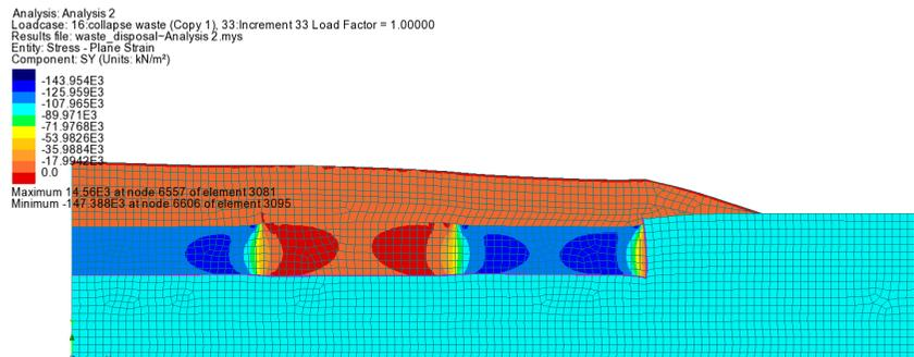
Figure 19: Vertical stress distribution after collapsing waste
