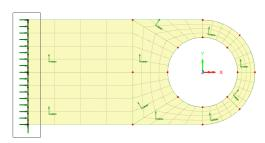
• Ensure the options to **Assign to lines** for **All analysis loadcases** are selected and click **OK** to finish assigning the support attribute.
