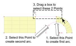
Thirdly, drag a box around the two unconnected points at the top of the model.
