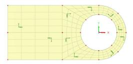
The axes of all surfaces can be aligned to axes of the first surface in the selection using the cycle relative facility.
