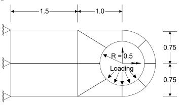
210E9 N/m<sup>2</sup>, a Poisson's ratio of 0.3 and a mass density of 7800kg/m<sup>3</sup>.
