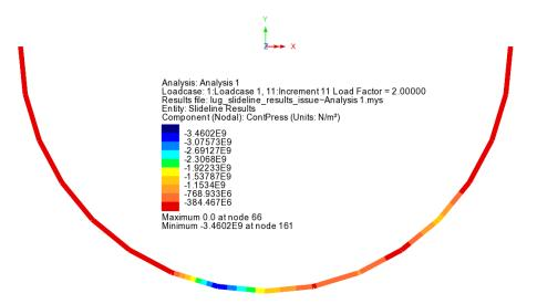
To plot a graph of the contact pressure distribution around the contact surface:
