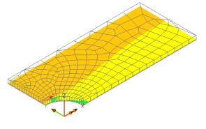
The contour key should be showing a maximum stress in the lamina X material direction of around 1.8E3
