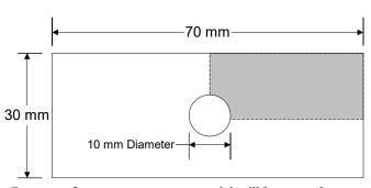
by a 10mm diameter hole. Because of symmetry a quarter model will be created.
