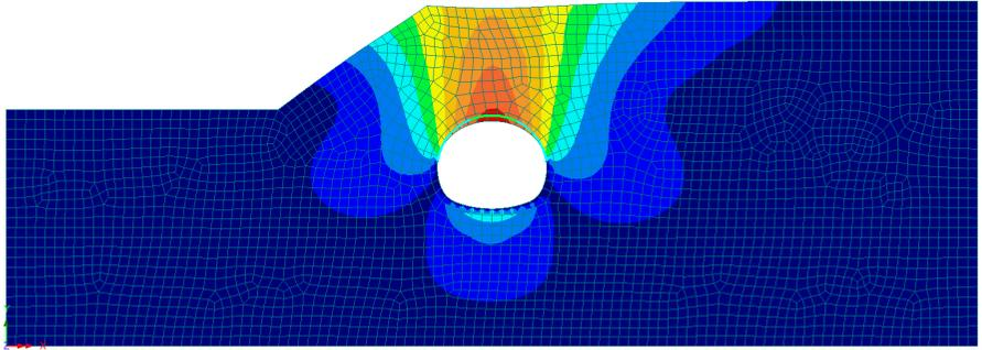
Figure 5: Resultant displacements at end of construction
