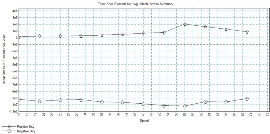
From the associated graph data table, the largest positive and negative peaks are seen to occur at a speed of 55m/s with values of 2.03Mpa and -10.2MPa respectively.
