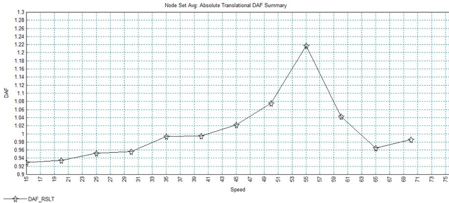
An envelope of the peak dynamic amplification factors for the selected nodes is displayed on screen in Notepad and written to the **Abs\_peak\_dafSet1.sum** which can be found in the \LUSASFiles32\IMDPlus\_rail\_bridge\IMDPlus\_Graphing folder.
