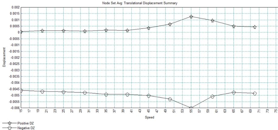
An envelope of the peak displacements and rotations for the selected nodes is displayed on screen in Notepad and written to the file **peak\_dspSet1.sum** which can be found in the \LUSASFiles32\IMDPlus\_rail\_bridge\IMDPlus\_Graphing folder.
