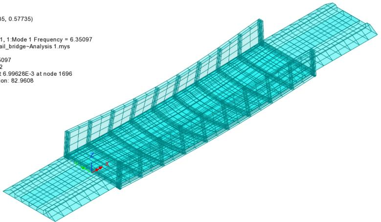
By setting each Eigenvalue to be active the deformed mesh can be seen for all mode shapes.
